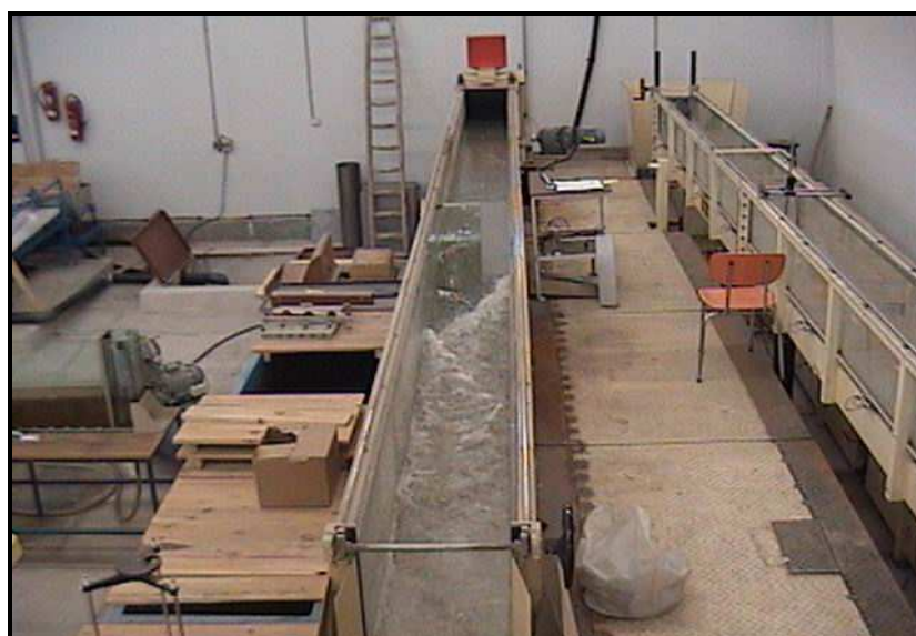
Figure 2. General view of the experimental setup and developed shocks
