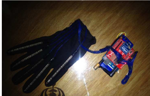
Fig. 14 Flex Sensor and Xbee based Transmission Side
