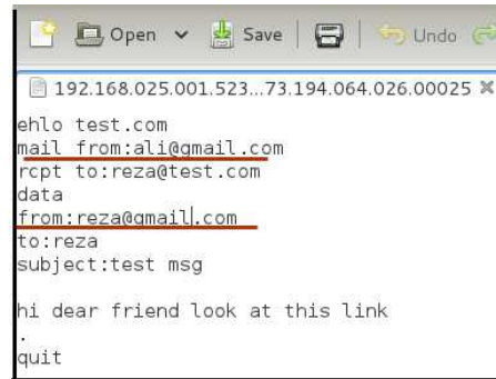
Fig. 2. Different sender fields in header and body
