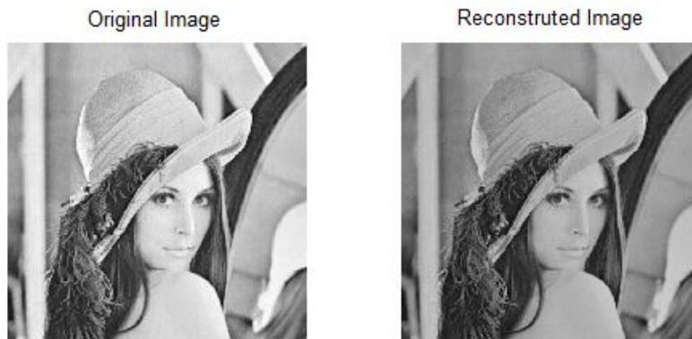
Figure 5. Results of proposed compression method for Lena image. PSNR=53.28, CR=2.09 and Filter: Coif1
