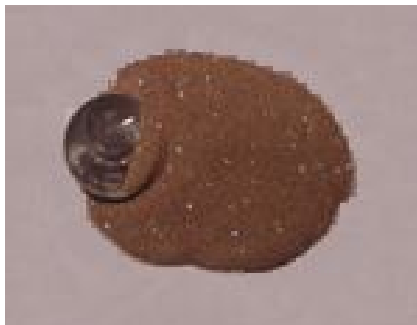
Figure 1.100 mesh zirconium sand ( ZrSiO_4 ), with the reddish chocolate colour. The copper-coloured coin is shown for colour comparison.
