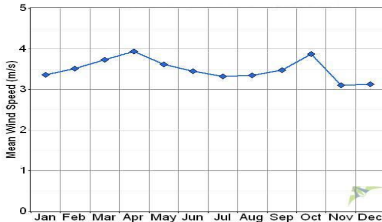
Figure 5: Average monthly speed of the wind during statistical period and in 10 meters height in Baladeh Station
