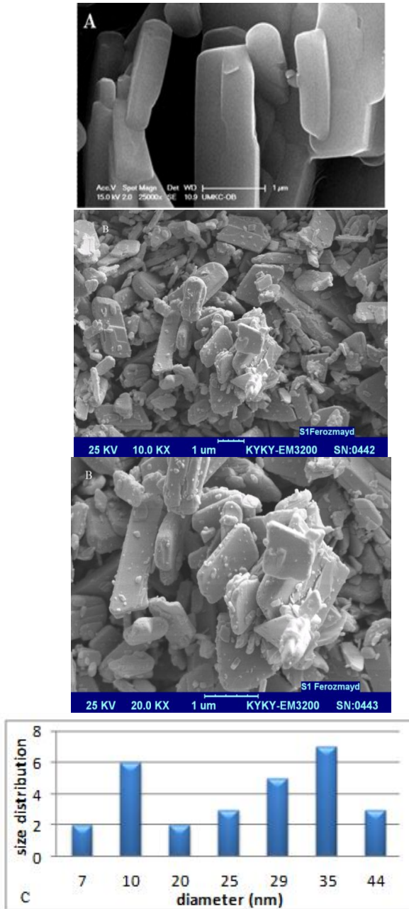
Fig. 3: SEM photographs of a) furosemide, b) furosemide nanoparticles (sample 2) and c) the particle size histogram of the nanoparticles.
