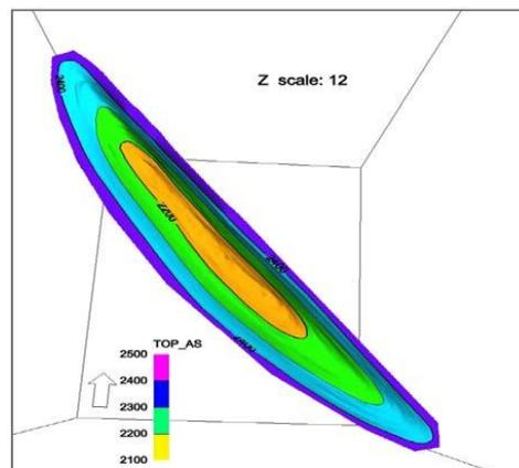
Figure 3: structural modelling of Mansuri field on the Asmari
