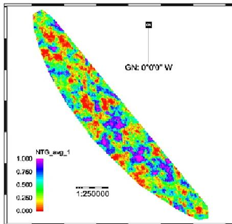
Figure 11: the normal distribution map for the net thickness over the entire zone 1
