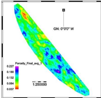
Figure 7: the normal distribution map for porosity zone of an Asmari
