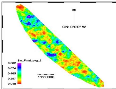
Figure 9: the normal distribution map for water saturation of zone 2 Asmari
