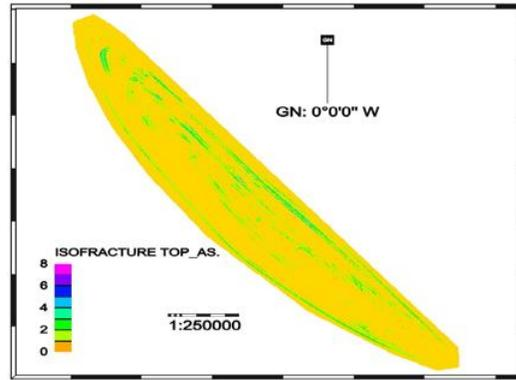
Figure 6: semi-breakage density map on the Asmari horizons
