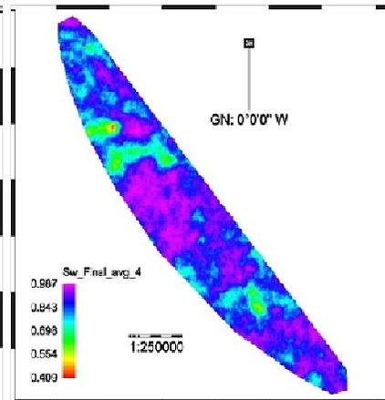
Figure 10: the normal distribution map for water saturation of zone 4 Asmari
