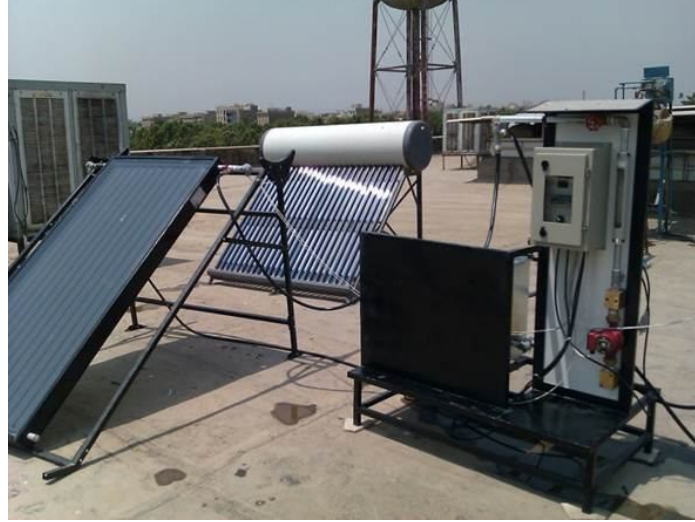
Fig.1. Collector test facility used for testing the collectors.
