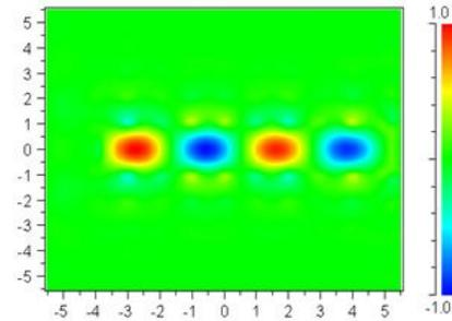
Fig. 4: Electric-field distribution of TE line defect (waveguide).
