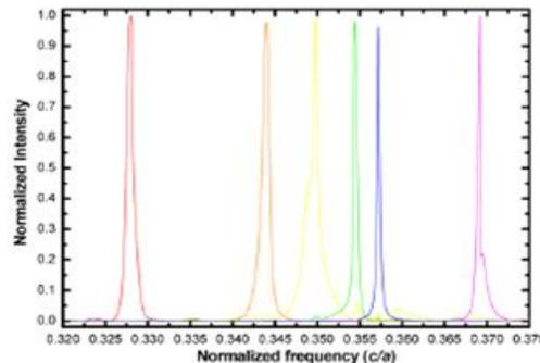
Fig. 4: (a) Schematic view of the proposed 5 channel drop filter, where channels are located on both sides of the bus waveguide the bus waveguide is terminated with another channel, in order to use the space more efficiently. The dielectric constant of all rods is  $11.56$ . (b) Transmission spectrum of the proposed filter, which has been calculated using the 2D-FDTD method.
