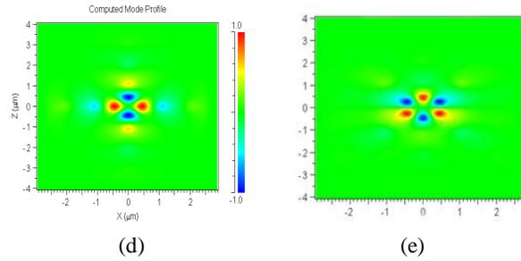
Fig. 3: The electric field distributions of the defect modes for a square array of dielectric rods in the air. (a) Monopole,  $R=0.10a$  (b) Doubly degenerate dipoles,  $R=0.33a$ . (c) monopole,  $R=0.60a$  (d) Second-order,  $R=0.60a$ . and (e) Doubly degenerate hexapoles,  $R=0.60a$ .
