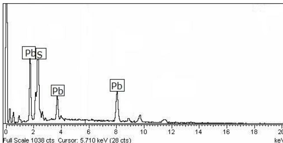
Figure 3: Energy dispersive X-ray analysis spectrum for the PbS films deposited at 75 °C
