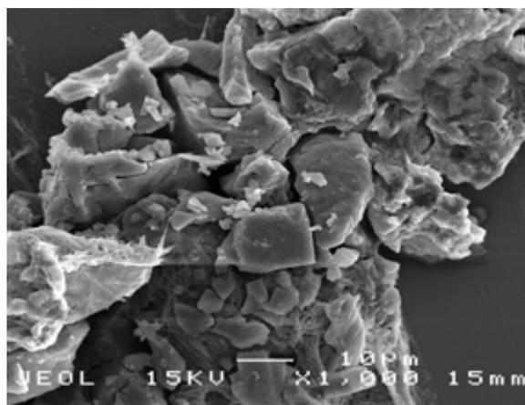
Figure 2: Scanning electron microscopy micrograph of the PbS films deposited at 75 °C
