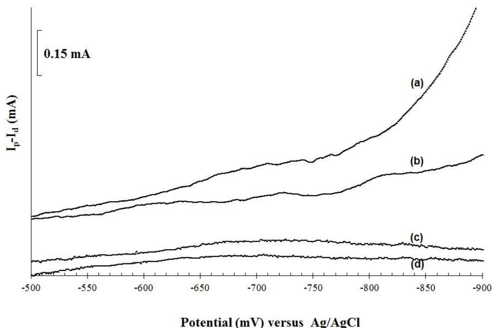
Figure 1: Comparison of photosensitivity of the PbS films deposited at different bath temperatures [a] 75 °C [b] 65 °C [c] 45 °C [d] 35 °C
