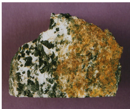
Fig. 4: Hornblende porphyroblasts and garnets in pargasite the small-grain plagioclase's mass.
