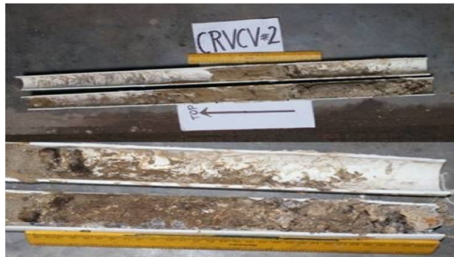
Fig. 13. Coral Boulders enriched Paleo Tsunami deposit observed from 31.6 to 64 cm overlain by very fine sand at Corbyn's Cove
