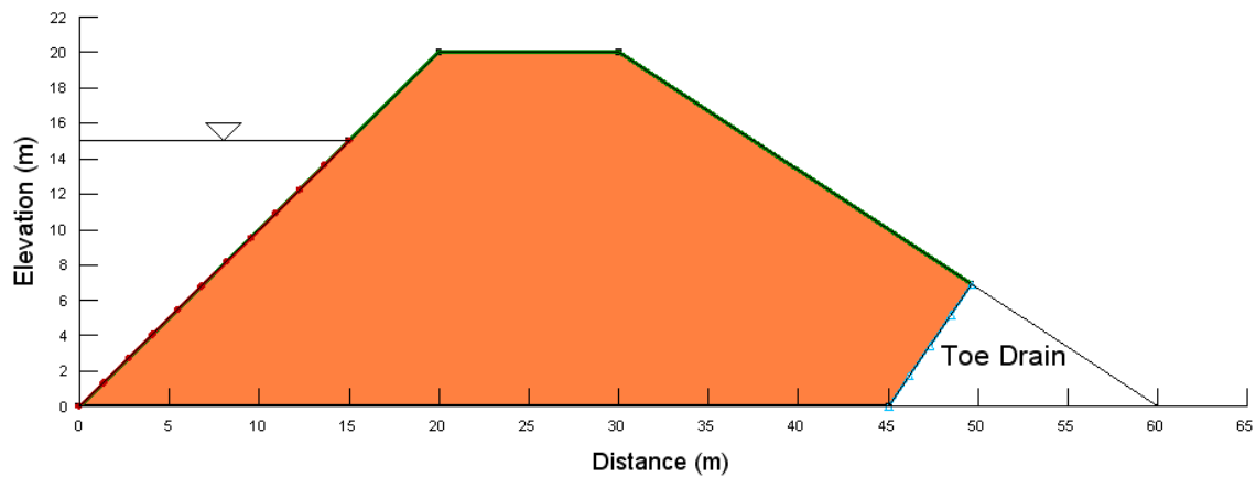
Figure 2. Geotechnical section of the dam.
