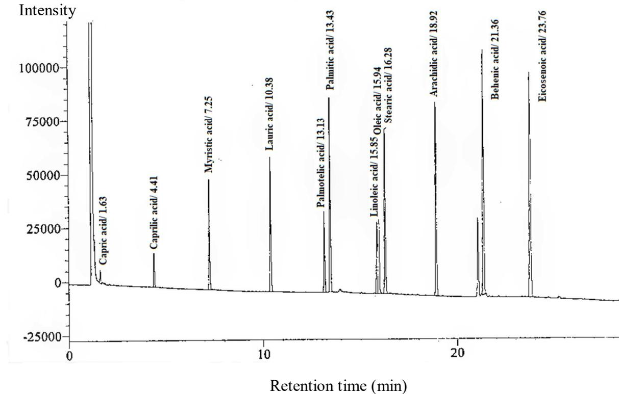
Fig 1. GC spectrum of standard fatty acid mixture
