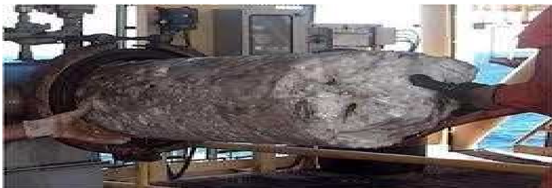
Figure 1: Developed gas hydrate plug in production line [6]
