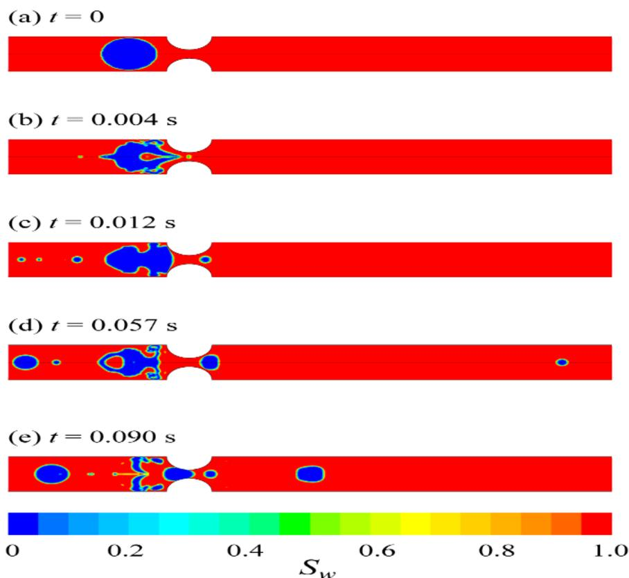
**Figure 3: Flow evolution during the continuous injection presented by volume fraction of water and oil phases during the first 0.090 s**
