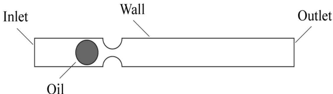
**Figure 1: Geometry of the 2D axisymmetric converging-diverging capillary tube model**
