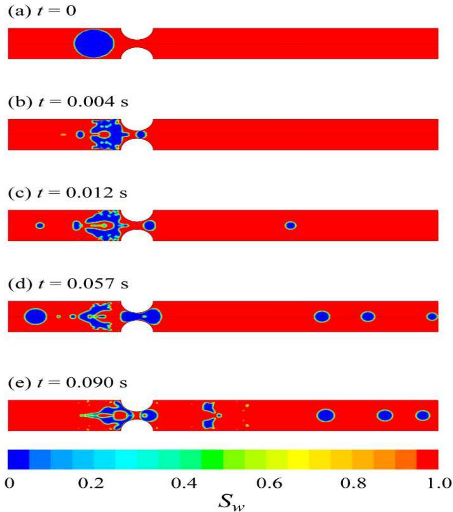
**Figure 4: Flow evolution during the pulsed injection presented by volume fraction of water and oil phases during the first 0.090 s**
