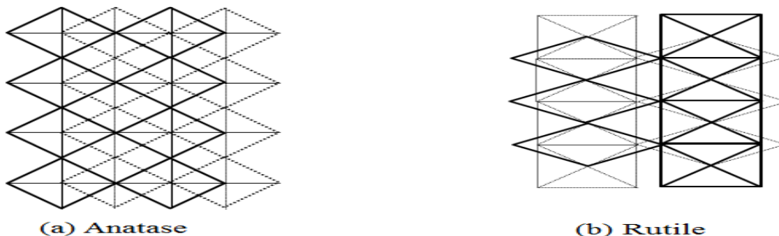
Figure 2: Two- dimensional projection of the TiO 6 octahedra along c-axis in (a) anatase and (b) rutile (the bold lines refer to shared edges) [4]
