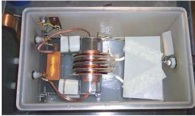
Fig. 3. Prototype CCPS HV tank including the 270:1 transformer, HV diode rectifier and HV feedback circuit.
